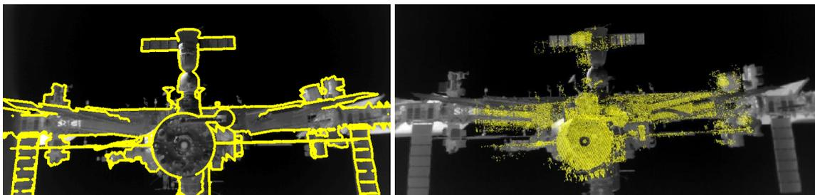
*Left. Example of ISS tracking in images, where the 3D model is accurately known a priori. Right. Example of LiDAR data acquired on the ISS. Both camera and LiDAR data have been acquired during the LIRIS experiment on ATV-5.*
