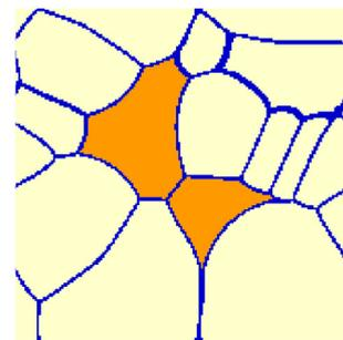
*Example of phase-field modeling of an austenite-to-ferrite transformation, 2D cut of a 3D simulation - (white) Ferrite grains - (orange) Austenite grains<sup>b</sup>*
